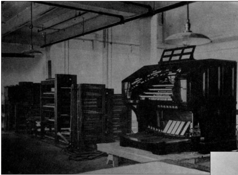
LEFT: Console, switchstacks, relays set up on erecting room floor of the Wurlitzer factory for tryout of instrument before it was shipped.
